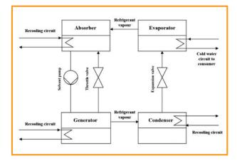
*Figure 6.13: Functional diagram of an absorption refrigerator*
