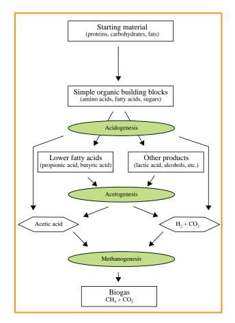
Figure 2.1: Schematic representation of anaerobic decomposition
