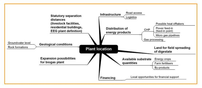
Figure 9.2: Parameters influencing the choice of plant location (CHP: combined heat and power)
