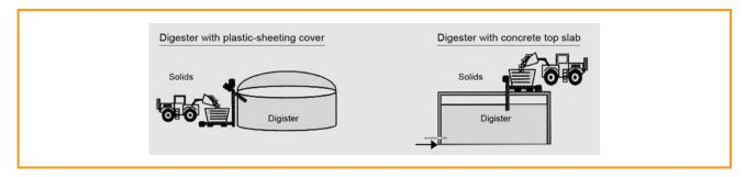
Figure 3.16: Direct solids infeed (schematic) [3-1]
