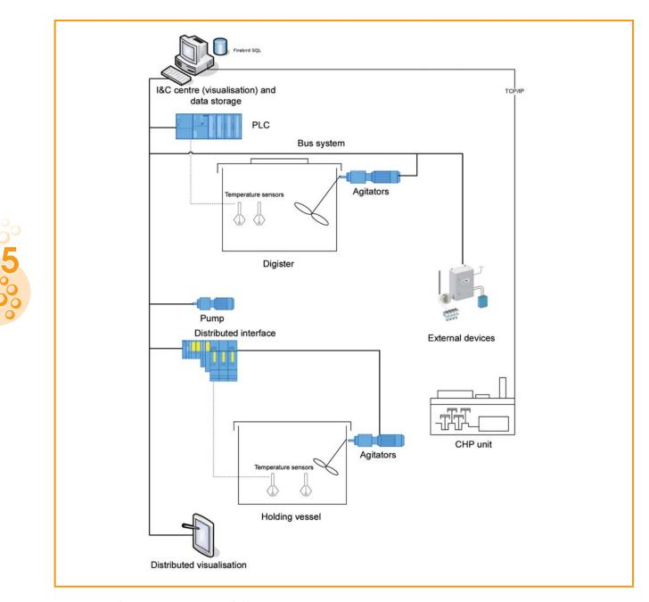
Figure 5.2: Schematic representation of plant monitoring
