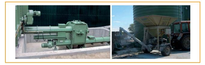
Figure 3.7: Beater and roller mill for comminuting solid substrates [Huning Maschinenbau GmbH, DBFZ]
