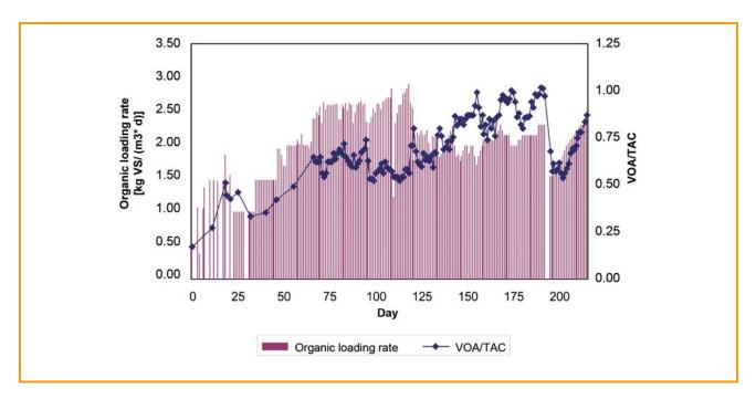
Figure 5.7: Progress of start-up phase of digester 1 with a deficiency of trace elements
