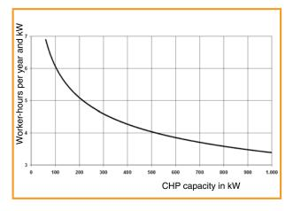
*Figure* 9.5: *Required working time for plant supervision and maintenance* [9-5]
