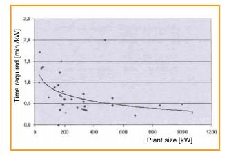
Figure 9.4: Required working time for plant supervision [9-4]
