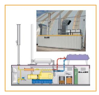
*Figure 6.5: Biogas CHP unit, compact stand-alone module with emergency flare [Haase Energietechnik AG]*
