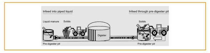
Figure 3.15: Indirect solids infeed (schematic) [3-1]
