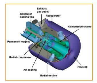
*Figure 6.11: Construction of a gas microturbine* [*Energietechnologie GmbH*]
