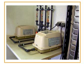
*Figure 6.1: Gas control system for injecting air into the digester gas space [DBFZ]*
