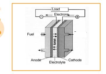
Figure 6.12: Operating principle of a fuel cell [vTI]
