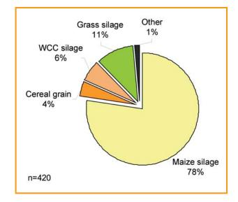
*Figure 12.6: Mass-based use of energy crops as substrate in biogas plants (operator survey 2009) [12-3]*
