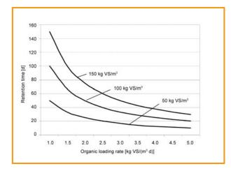
*Figure 2.2: Correlation between organic loading rate and hydraulic retention time for various substrate concentrations*
