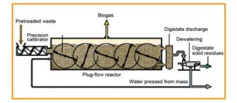
*Figure 3.24: Plug-flow reactor (dry digestion) [Strabag-Umweltanlagen]*
