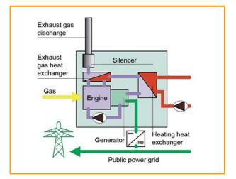
Figure 6.4: Schematic layout of a CHP unit [ASUE]
