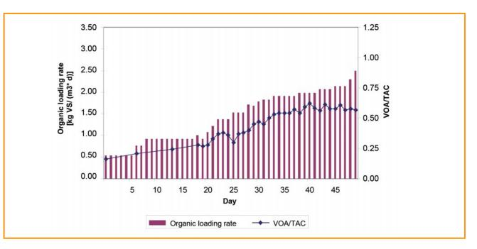
Figure 5.5: Progress of start-up phase, digester 2
