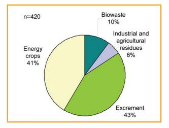
*Figure 12.5: Mass-based substrate input in biogas plants (operator survey 2009) [12-3]*
