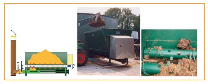
Figure 3.18: Infeed of stackable biomass into the digester with ram feeder [PlanET Biogastechnik GmbH]
