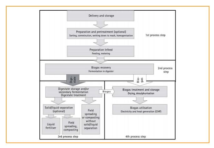
Figure 3.3: General process of biogas recovery; as described in [3-3]
