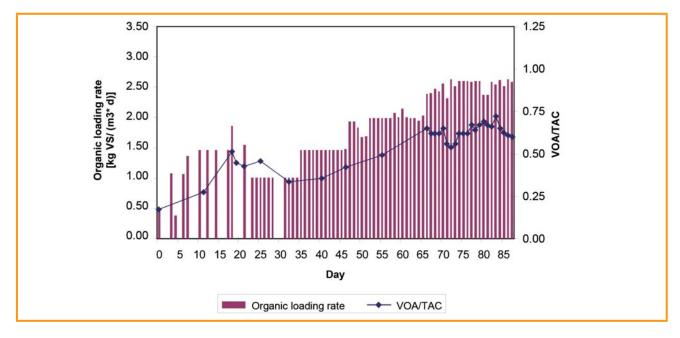
Figure 5.4: Progress of start-up phase, digester 1
