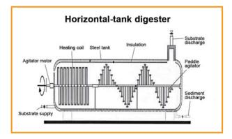
Figure 3.23: Plug-flow reactor (wet digestion) [3-4]
