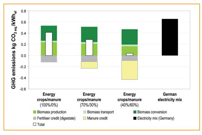
*Figure 12.2: Greenhouse gas emissions (kg*  $CO_{2 eq}/kWh_{el}$ ) from model biogas plants compared with German electricity mix [12-5]
