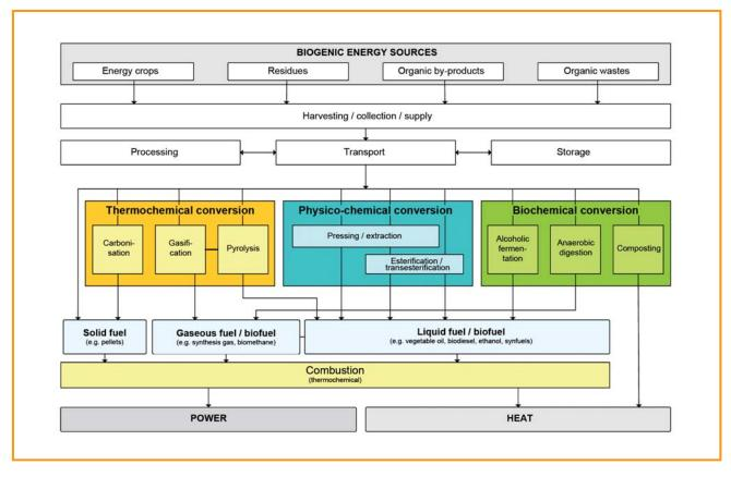
Figure 12.1: Options for utilising biomass for the supply of final energy/useful energy
