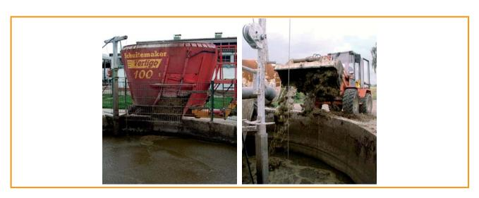
Figure 3.14: Pre-digester or receiving pit in feeding [Paterson, FNR; Hugo Vogelsang Maschinenbau GmbH]
