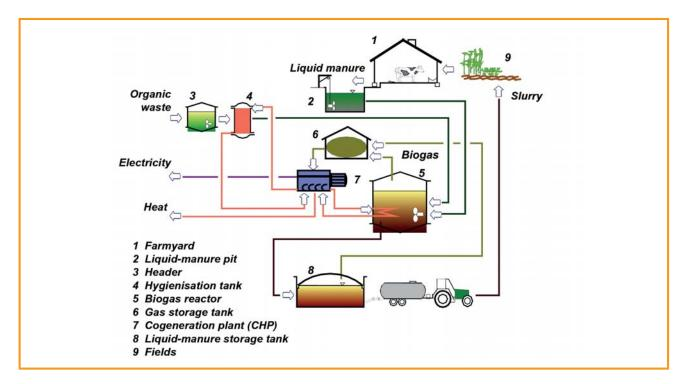
Figure 3.4: Schematic of an agricultural biogas recovery plant for co-substrates [ATB]
