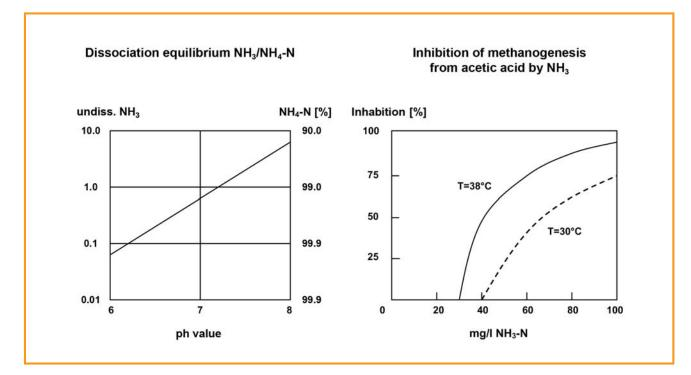
Figure 5.1: Inhibition of methanogenesis from acetic acid by NH<sub>3</sub> (as per [5-2])
