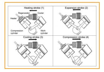
*Figure 6.10: Operating principle of a Stirling engine from* [6-14] according to [6-21]
