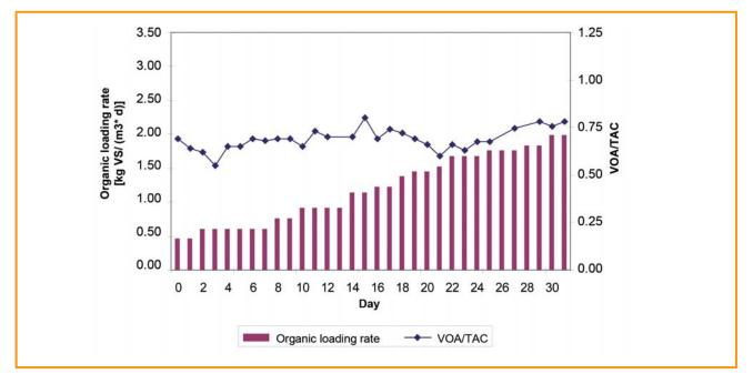
Figure 5.6: Progress of start-up phase, digester 3
