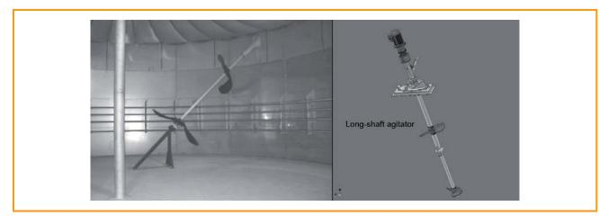
*Figure 3.32: Long-shaft agitators with two stirring blades with and without shaft-end bearer on the bottom of the digester [WELtec BioPower GmbH; graphic: Armatec FTS-Armaturen GmbH & Co. KG]*
