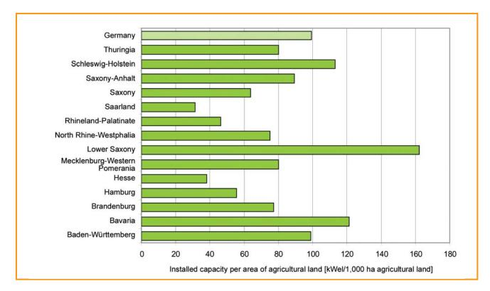
*Figure 12.4: Installed electrical capacity in relation to the area of agricultural land*  $[kW_{el}/1,000$  *ha agricultural land] in the German federal states (based on data from [12-3], [12-6])*
