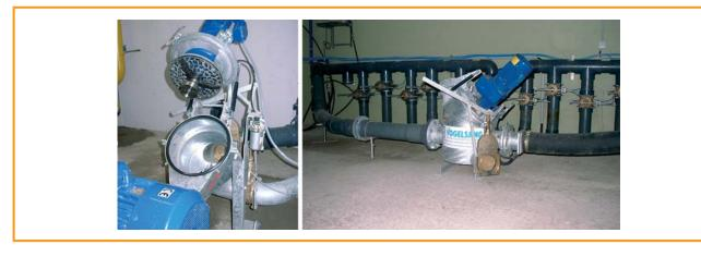
Figure 3.8: In-pipe substrate comminution (perforated-plate comminutor) [Hugo Vogelsang Maschinenbau GmbH]
