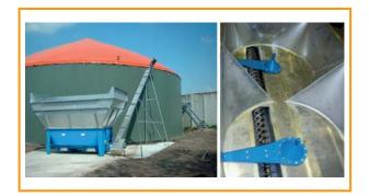
Figure 3.6: Receiving vessel with loosener [Konrad Pumpe GmbH]
