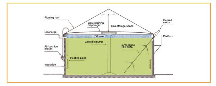
Figure 3.22: Stirred-tank reactor with long-shaft agitator and other internals [Anlagen- und Apparatebau Lüthe GmbH]
